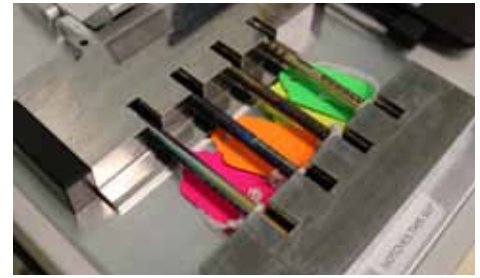
Chemicals from participants’ breath are captured in small metal tubes and sent to Picomole for analyzing.
